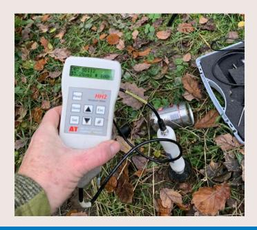
We installed eighteen forty centimetre long tubes into the ground either side of a hedge in a known flood pathway in Wilderness Meadows to begin measuring soil moisture at ten, twenty, thirty and forty centimetres depth as well as at ground level using specialist equipment. Measurements will be taken over the next 18 months as a scientific experiment to try to determine whether hedges do slow the flow and help mitigate flooding.
